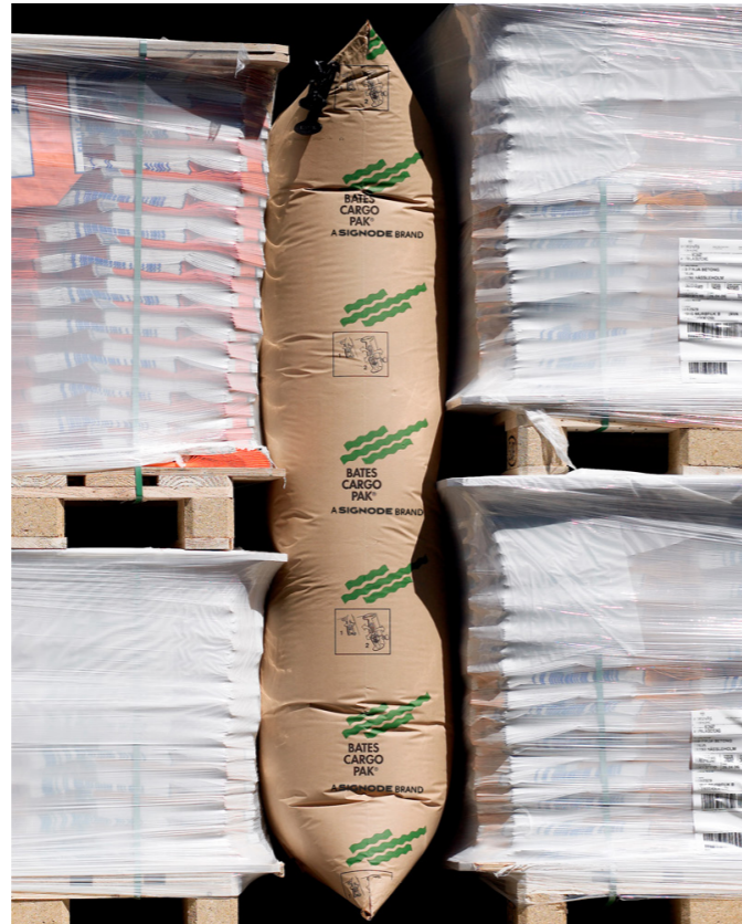
Reuse airbag inflated in position
