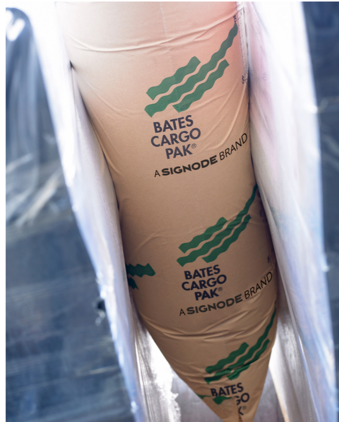
Flex airbag inflated in position
